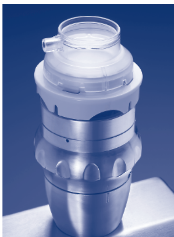
2. Access the membrane by connecting the MSOpener™ to a vacuum source, and placing the MicropreSure On-Line Filtration Sampler on top of the MSOpener.
